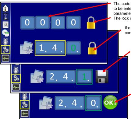
The code or diagnostics plug for setting parameters does not have to be entered or connected if the operator wants to adjust parameters (only released parameters can be adjusted). The lock is locked.
