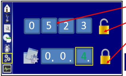
If parameters are to be changed, the code for setting parameters must be entered (alternatively, diagnostics plug).
